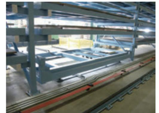
● Loading and unloading electric cart
