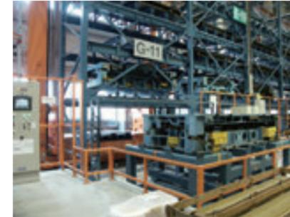
● Loading and unloading station of 40,000-ton press machine molds
